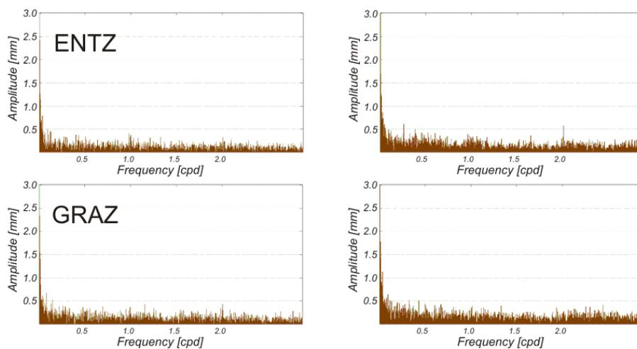
**Fig. 5** Periodograms of sites without significant oscillation (less than 1 mm), left: N-S component, right: E-W component.
