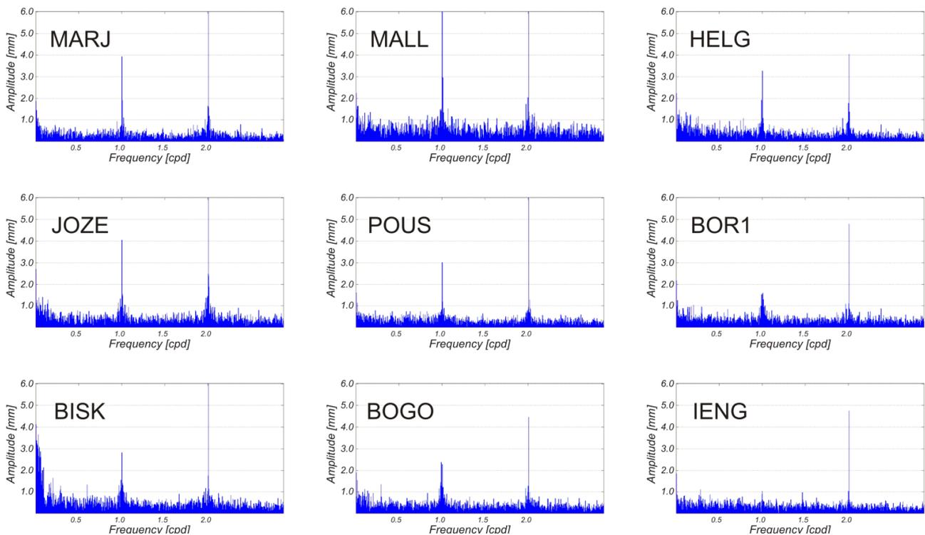
**Fig. 3** Periodograms of sites with oscillations in height component (amplitude higher than 3 mm).
