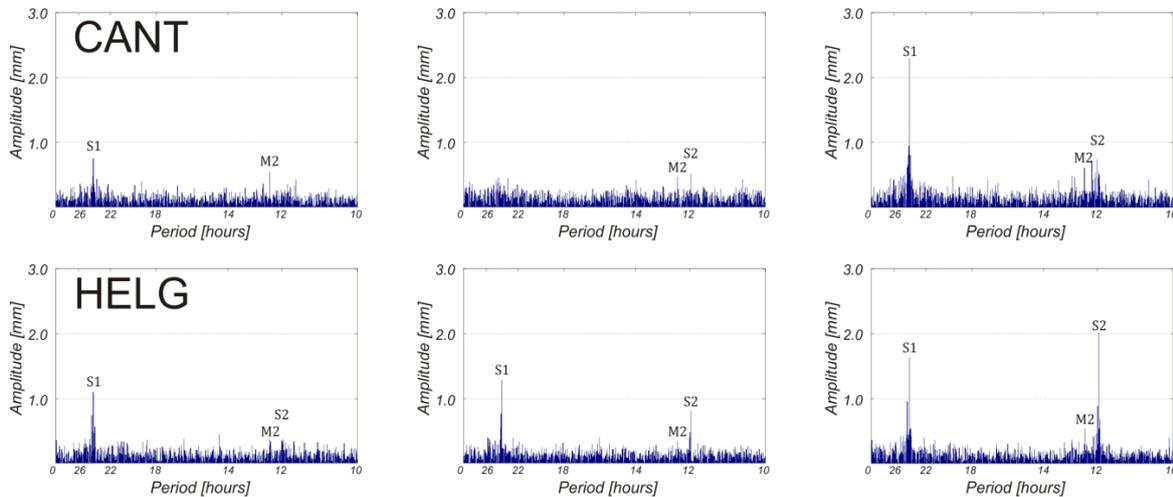
**Fig. 10** Periodograms of coastal sites with oscillation in M2 frequency (from left: N-S component, E-W component, height ).
