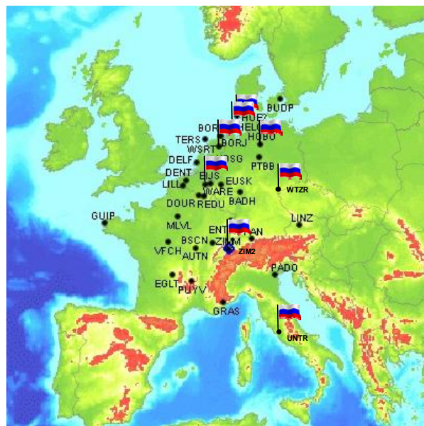
Figure 1: Eight sites of the EPN subnetwork processed by swisstopo providing combined GPS/GLONASS data (BORJ, EIJS, HELG, HOBU, HOE2, UNTR, WTZR, ZIM2).
